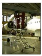
1 or 2 person lift and capacity spring assisted maintenance platform. Multiple height positions. Locking wheels. Removable handrails. Deck end or side extension ladder entry. Ladder may stow under deck when platform folded flat. Deck sizes to 6' x 40", outrigger & telescoping legs, tool trays, deck padding. Canadian made. CSA, ANSI & Osha compliant.
